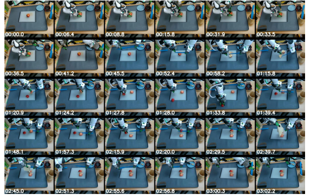
(b) Frames from a successful rollout for the CutAppleInSlices task on wood_island . This is the longest horizon task in our benchmark, and it can take up to 3 minutes to complete. The robot has to first use a tool to remove the core of the apple, after which, using a knife, it has to first slice the apple in half, position each half in the workspace and slice at least one half in at least 3 slices. Finally, the robot has to wipe the knife with a cloth, put it in the sheath, and place is back into the utensil crock.
