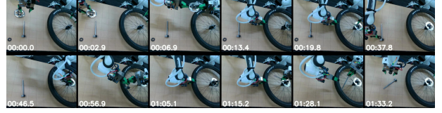
(a) Frames from a successful rollout for the BikeRotorInstall task on ruggles . This task requires a high degree of precision, as well as bimanual coordination: while holding the wheel down with one arm, the robot has to place a rotor and a locking onto the wheel as well as manipulate a tool with which to tighten the locking for at least one revolution of the tool around the center axle of the wheel.
